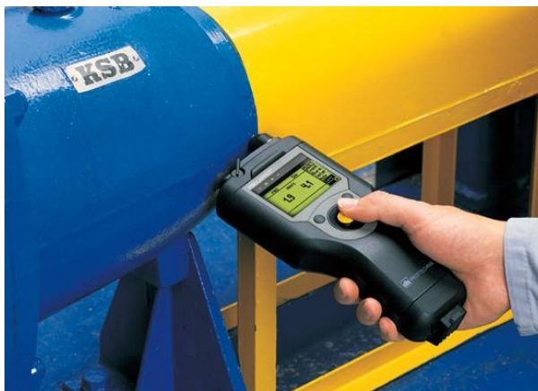
VIBSCANNER – a typical low cost portable CM system
