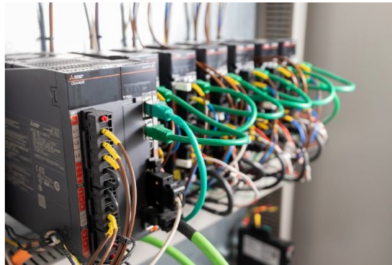
Figure 4: The setup includes Mitsubishi Electric's Melsec MR-J5 servos controlled by an iQ-R series PLC, A which are all compatible with CC-Link IE TSN. Courtesy: CC-Link Partner Association (CLPA)
