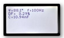
capacitance measurements) is the measure of the dielectric (insulating) losses in an electrical insulating material in an alternating (current) field and the resulting energy dissipated as heat. DF is used as a means of measuring changes in MGU phase winding
